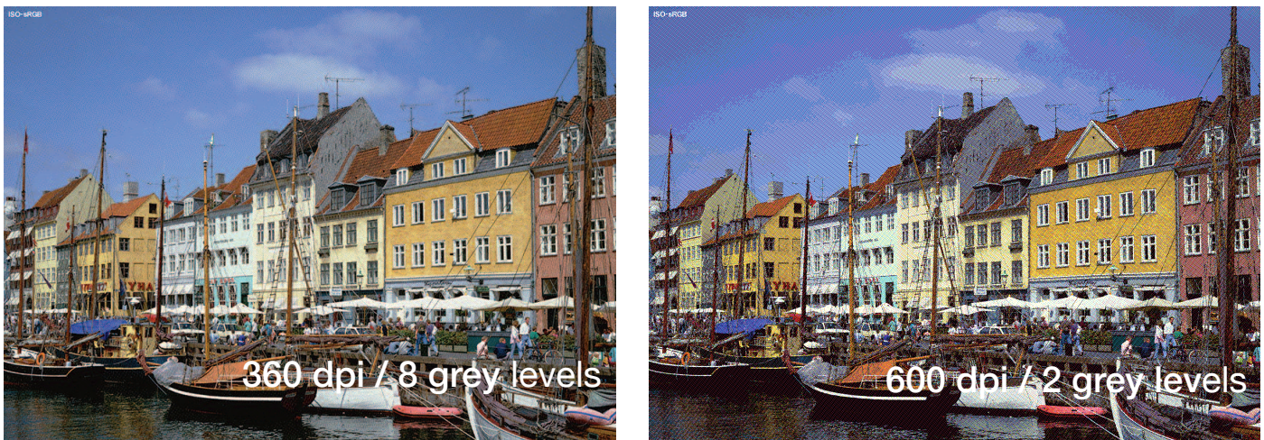
Figure 8: Digital image simulation of 360 dpi with 8 grey levels compared to 600 dpi with 2 grey levels
