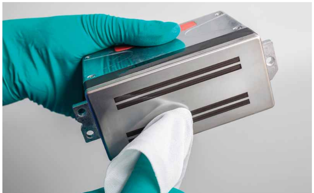
Figure 7: If manual cleaning is required, wipe the printhead ONCE and in ONE direction with a clean lint-free cloth.
