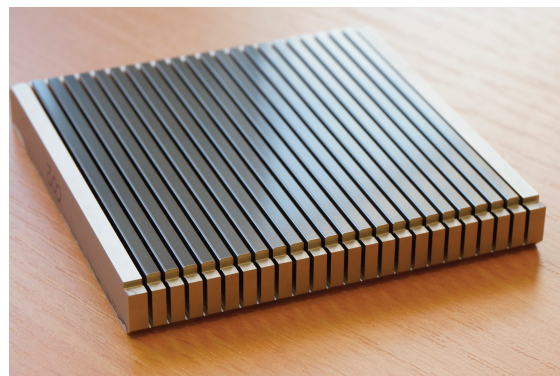
Figure 5: Edge-shooter wafer assembly prior to separation
