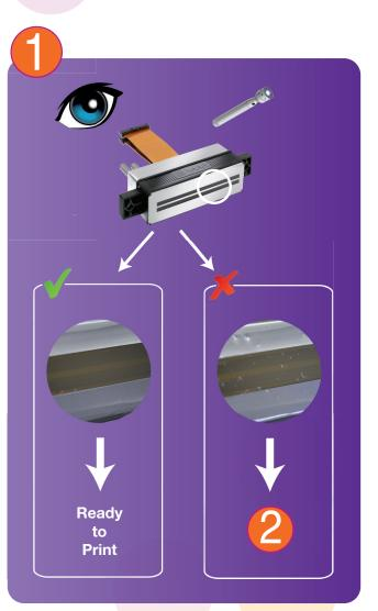
Detailed below is the procedure for cleaning contamination from the printhead. Always use the correct method for wiping the nozzle plate.
