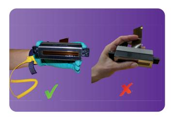
Do NOT touch the sensitive parts of the printhead. Always protect the printhead from static damage and wear gloves at ALL times.
