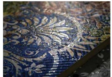
Ceramic tile gloss effect printed by Scientifica Tiles LLP, India at 60 g/m<sup>2</sup> at 24 m/min with Xaar 2001+ GS12 printheads using Xaar's High Laydown Technology
