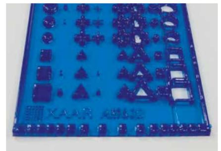
2.5D resolution test sample made with photopolymer (40 mPa.s @ 50C) printed using Xaar 1003 GS12 printhead with standard three-cycle jetting
