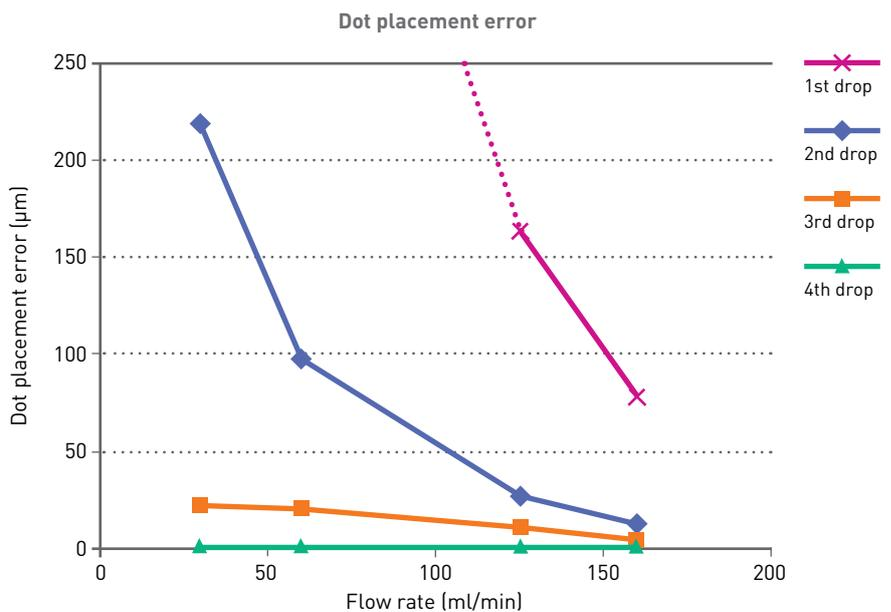
**Figure 8** shows that, at longer idling times, a flow rate of 125 ml/min prevents the loss of any drop. The first drop is ejected even after an idling time of 24 hours. The dot placement errors of the first drop increase in line with increased idling time, indicating the formation of a more viscous skin, whilst the second and third drops essentially have the nominal velocity.
