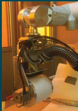
A Xaar jetting test rig with a Stäubli robot arm (at the Iprint Institute for Printing, Switzerland) is shown on the left with the close-up on the right showing a Xaar 1003 printhead mounted on the robot arm for jetting at high levels of acceleration and deceleration<sup>11</sup>
