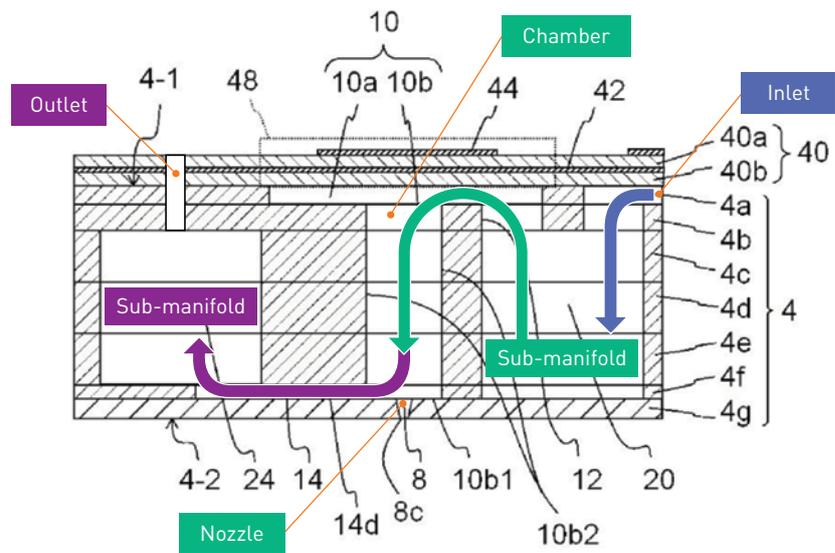
Another feature apparent in **Figure 3** is the narrowness of the ink inlets and outlets. There is a reason for this: by limiting pressure loss through the inlets and outlets, energy loss through the nozzle is reduced. However, the disadvantage is that because the overall flow path is restricted, the recirculation flow rate is necessarily much lower.
