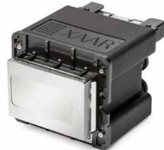
The Xaar 1201 is a Thin Film Piezo Silicon Micro Electrical Mechanical System (MEMS) technology printhead for printing Wide-format graphics and textiles which jets aqueous or ECO solvent inks. It has 1280 nozzles arranged in 4 rows printing either 2 colours at 600 dpi or 4 colours at 300 dpi native resolution.
