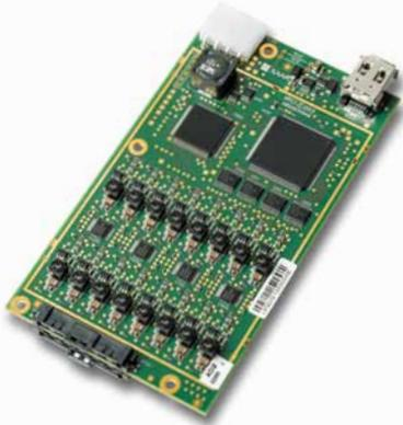
The Xaar HPCs provide optimal and dependable data communication between Xaar's printheads and the remainder of the digital inkjet print data path.
