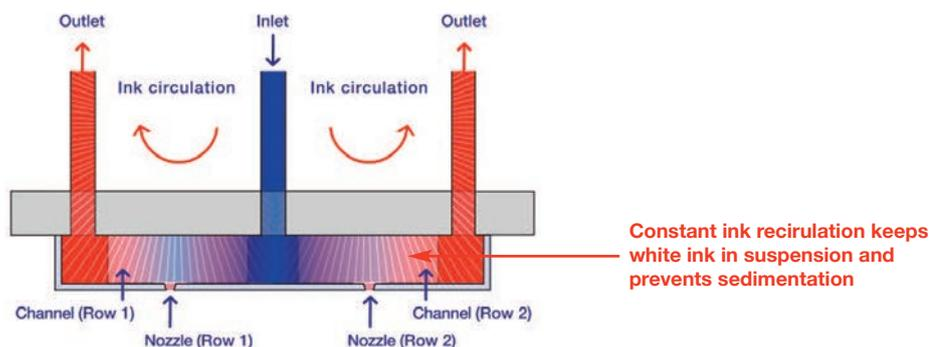
**Figure 6:** Constant ink recirculation prevents ink sedimentation and consequential nozzle blocking
