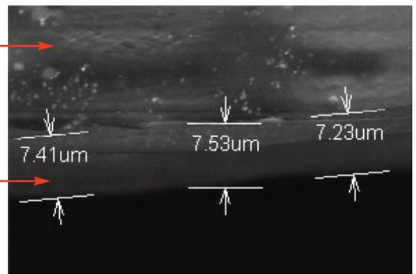
Figure 8: White ink film printed with single printbar
