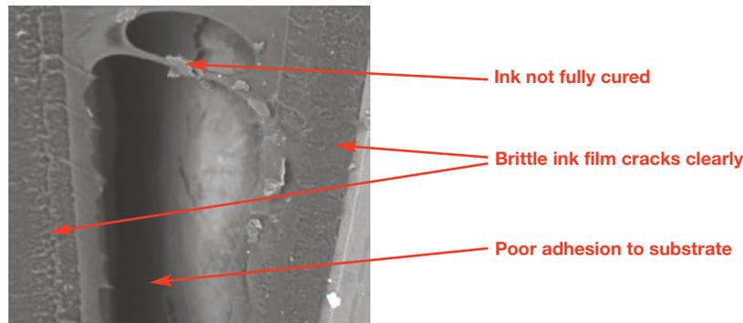
**Figure 11:** Opaque white ink printed with double printbar (non-Xaar printheads – 500x magnification)
