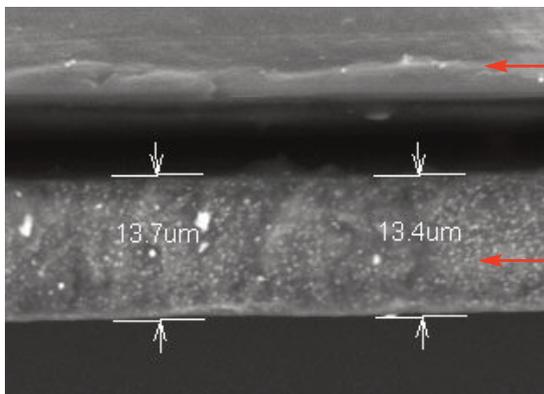
Figure 7: White ink film printed with double printbar
