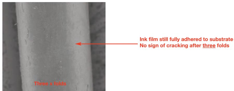
**Figure 9:** 8 µm ink film printed with single printbar of Xaar 1002 GS6 (200x magnification)
