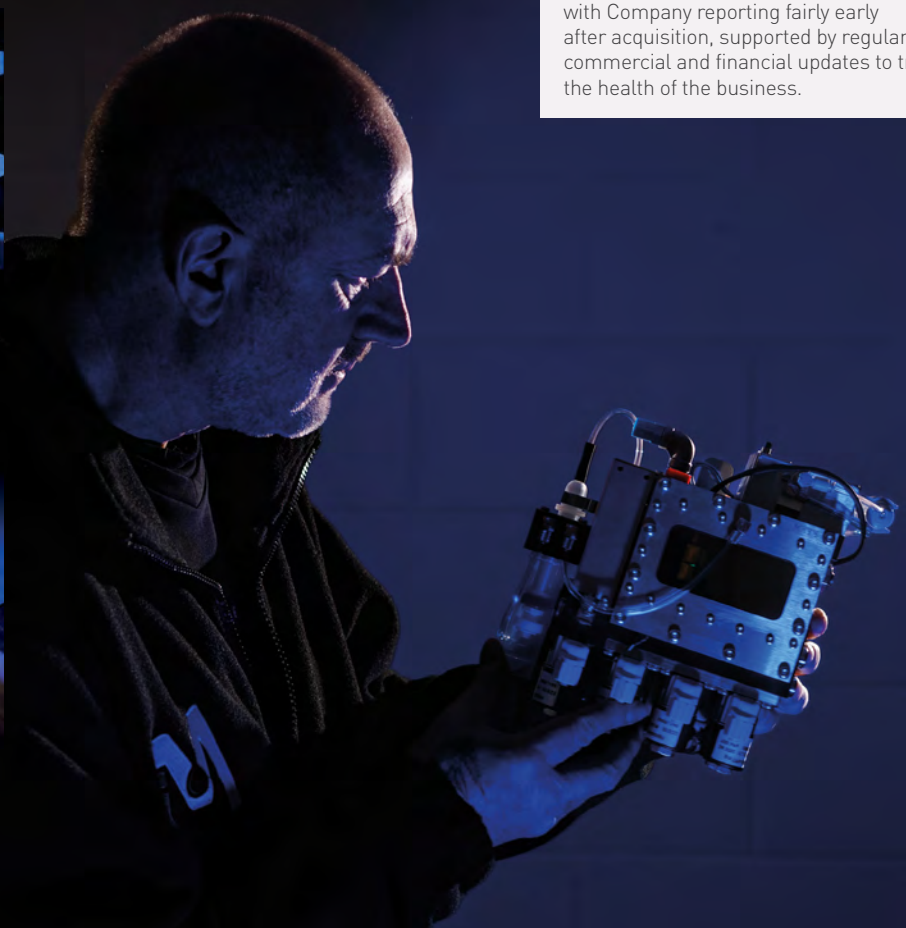
Labjet Gravity is a syringe-based gravity fed fluid management system, ideal for evaluating small volumes of fluids in a laboratory environment with industrial components.
